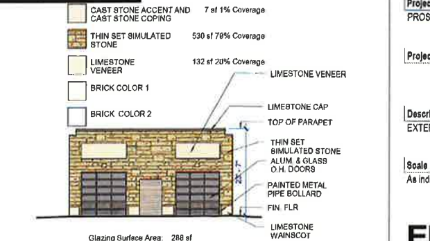
6 WEST SOUTH CARWASH ELEVATION SCALE: 1/16" = 1'-0"
