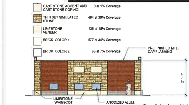
NORTH CARWASH ELEVATION SCALE: 1/16" = 1'-0"
