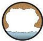
The start of a blocked pipe begins when grease and solids collect on the top and sides of the pipe interior.
