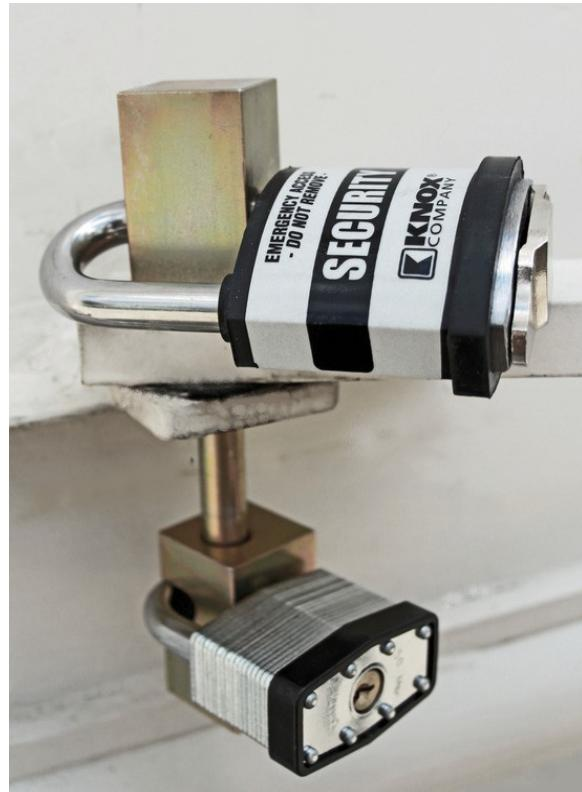
Place the other block on the pin and secure with a Knox™ Padlock.
