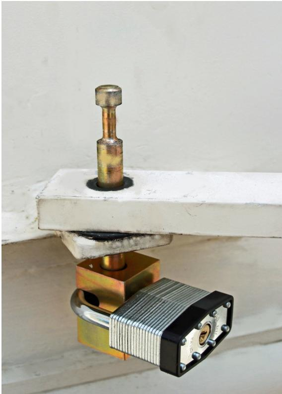
Secure the bottom block with a 3/8" diameter and a 1" x 1" shackle padlock. Insert the other end of the pin-up through the gate bracket and the swing gate arm.
