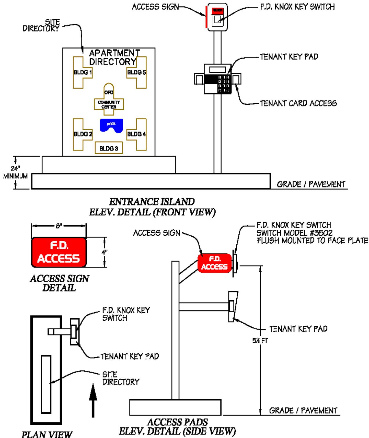
Figure 3 - Exit Only Sign Diagram with FD Access
