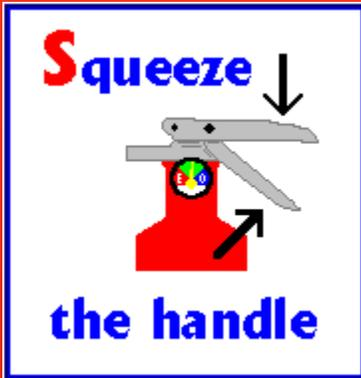
Squeeze the top handle or lever. This depresses a button that releases the pressurized extinguishing agent in the extinguisher.
